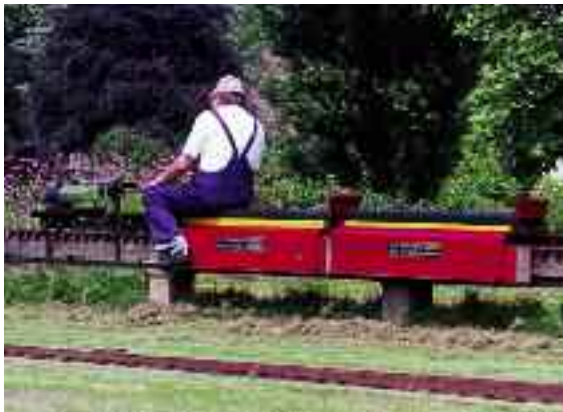
Elevated track passenger carriages showing valances and flexible coverings between the top and sides of the vehicles
